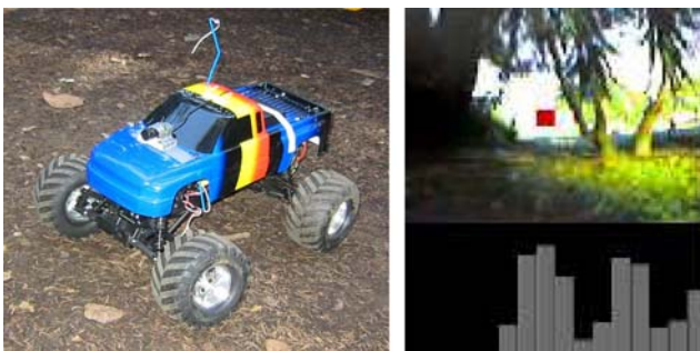
Fig. 11 a The remote-controlled car driven autonomously in various cluttered unconstrained environments, using our algorithm. b A view from the car, with the chosen steering direction indicated by the red square; the estimated distances to obstacles in the different directions are shown by the bar graph below the image
