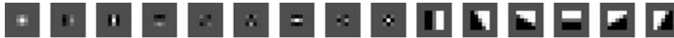
Fig. 2 The convolutional filters used for texture energies and gradients. The first nine are 3 \times 3 Laws' masks. The last six are the oriented edge detectors spaced at 30^\circ intervals. The nine Laws' masks are used to perform local averaging, edge detection and spot detection
