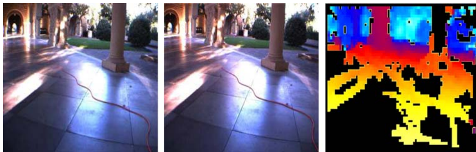
Fig. 12 Two images taken from a stereo pair of cameras, and the depthmap calculated by a stereo system
