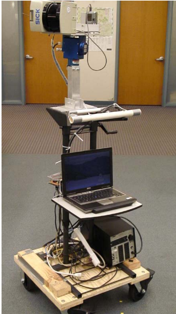
Fig. 7 The 3-d scanner used for collecting images and the corresponding depthmaps
