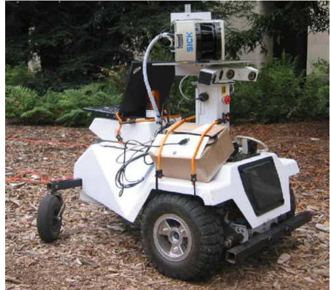
Fig. 8 The custom built 3-d scanner for collecting depthmaps with stereo image pairs, mounted on the LAGR robot
