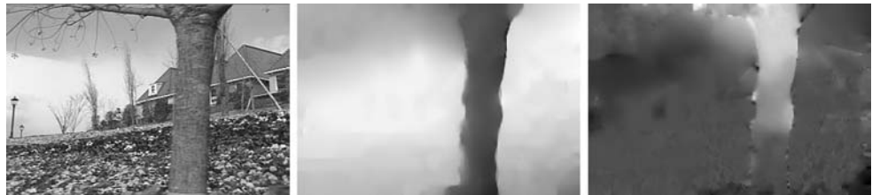
Fig. 12 Flower garden sequence: First image ( left ). Optical flow computed by the 2D affine over-parametrization model, u ( middle ) and v ( right )
