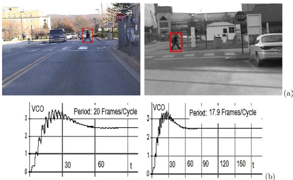
Figure 13. PLL output voltage vs. locking time for color/gray sensor. (a) Representative frames. (b) VCO output.
