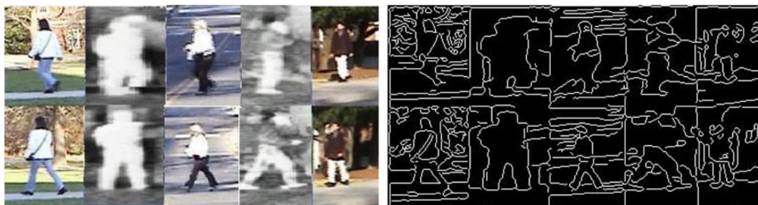
Figure 9. Principle Gait Angle in original and gradient images. Only those with MPGA exhibit a salient angle pattern.
