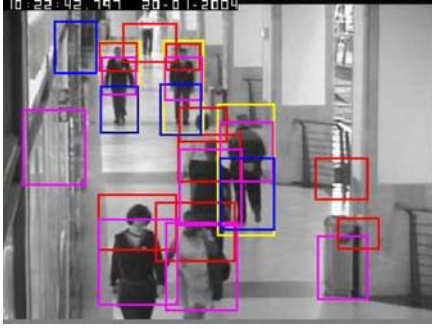
Figure 9. Part detection responses (yellow for full-body; red for head-shoulder; purple for torso; blue for legs).
