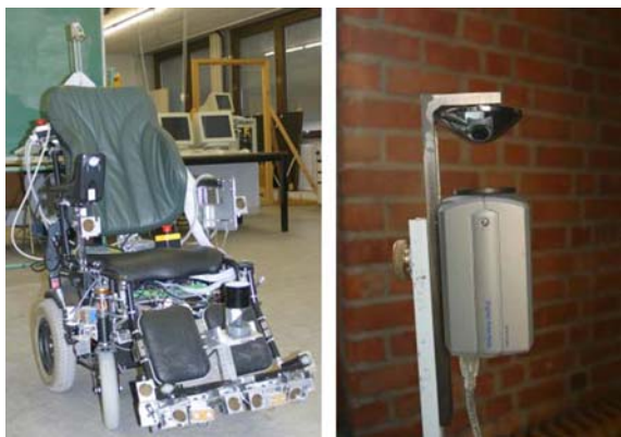
Figure 1. Left: the robotic wheelchair platform. Right: the omnidirectional camera, composed by a colour camera and an hyperbolic mirror.
