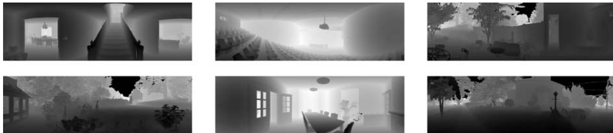
Figure 3. Example range scenes from the Brown range image database (Lee and Huang, 2000). Intensity here codes for depth with distant objects appearing brighter. Regions for which no range estimate could be obtained are shown in black.
