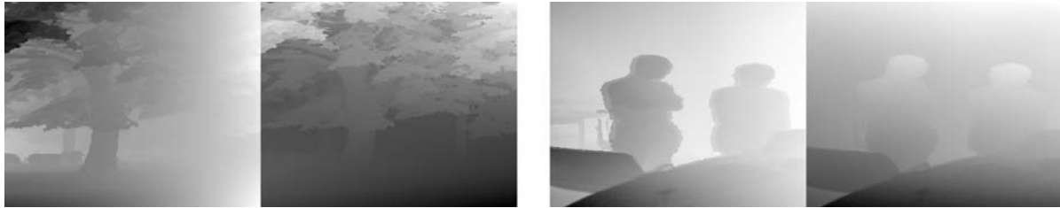
Figure 1. Flow fields generated for an outdoor (left) and an indoor (right) scene. The horizontal motion \mathbf{u} is shown on the left, the vertical motion \mathbf{v} on the right of each figure; dark/light means negative/positive motion (independently scaled to 0 \dots 255 for display).
