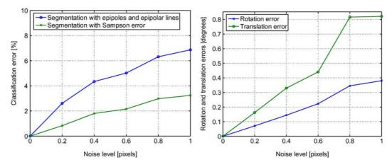
Figure 5. Percentage of correct classification and error in the estimation of rotation and translation (in degrees).
