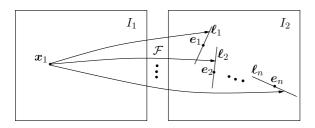
*Figure 3.* The multibody fundamental matrix  $\mathcal{F}$  maps each point  $x_1$  in the first image to *n* epipolar lines  $\ell_1, \ldots, \ell_n$  which pass through the *n* epipoles  $e_1, \ldots, e_n$  respectively. One of these epipolar lines must pass through  $x_2$ .
