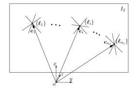
*Figure 4.* When *n* objects move independently, the epipolar lines in the second view associated with each image point in the first view form  $n_e \leq n$  groups intersecting respectively at  $n_e$  different epipoles (up to scale) in the second view.
