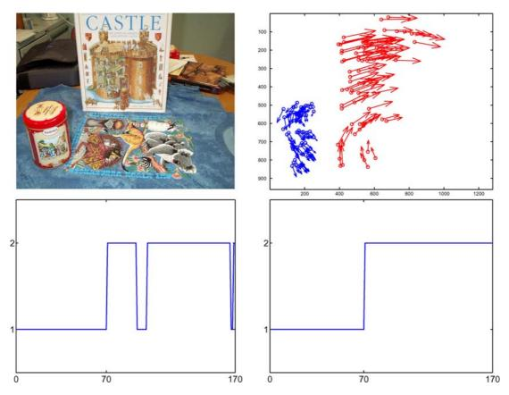
*Figure 6.* Top: first frame of a sequence with two rigid-body motions—the can and the background—and the 2-D displacements of the 140 correspondences from the first view ('o') to the second (' $\rightarrow$ '). Bottom: segmentation of the 170 correspondences using epipoles and epipolar lines (left) and using Sampson distance (right).
