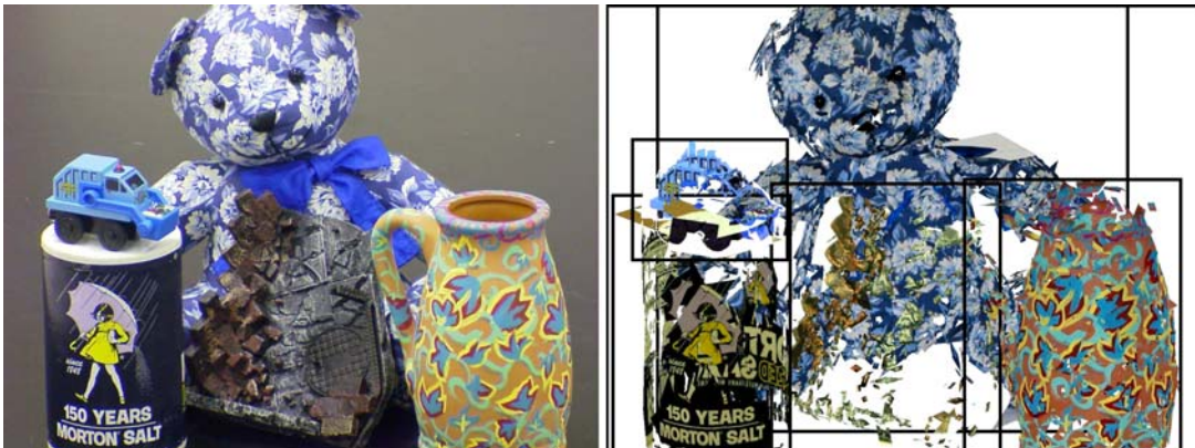
Figure 1. Results of a recognition experiment. Left: A test image. Right: Instances of five models (a teddy bear, a doll stand, a salt can, a toy truck and a vase) have been recognized, and the models are rendered in the poses estimated by our program. Bounding boxes for the rejections are shown as black rectangles.
