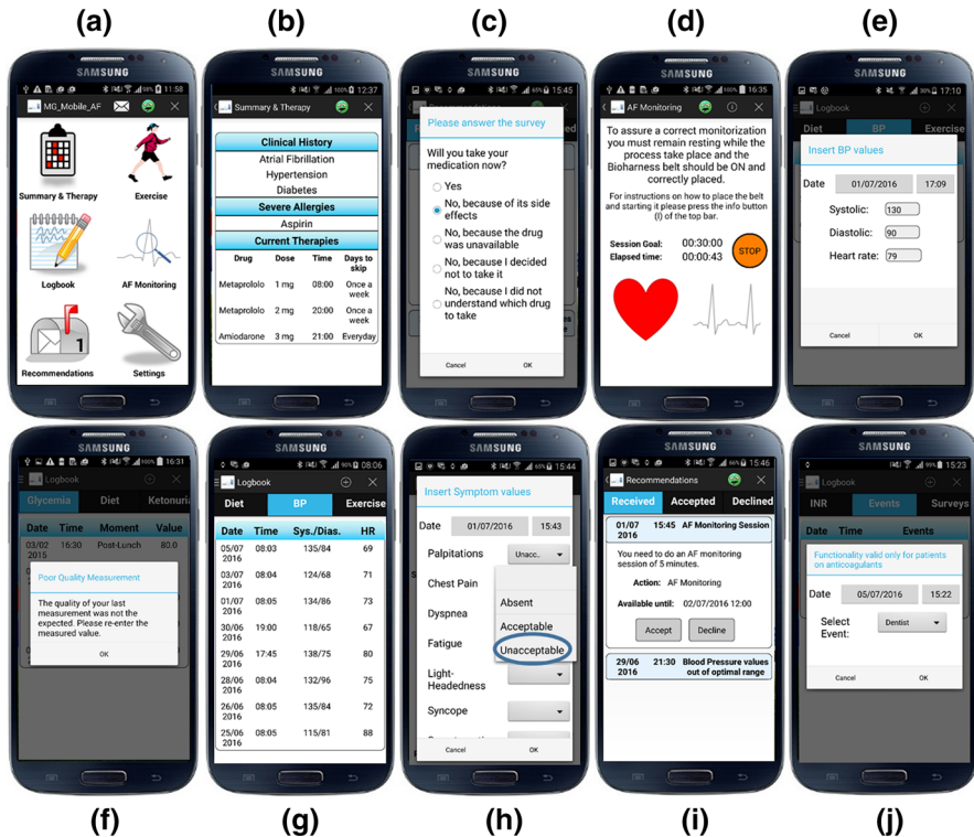
Fig. 2 MobiGuide patient UI. a regular first screen for Atrial Fibrillation (AF) (the Gestational Diabetes Mellitus [GDM] screen does not include the AF Monitoring icon); b active prescriptions; c medication reminders with a place to indicate non-compliance with reason; d ElectroCardioGram (ECG) monitoring screen; e logbook with Blood Pressure (BP) data entry; f bad quality of data message; g visualizing BP records; h selecting palpitations level; i recommendation to measure ECG due to symptom reporting; j informing the system of risky events (in this case risk of bleeding)
