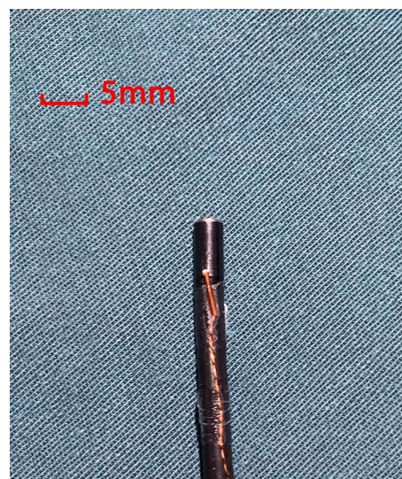
Fig. 1 The medical temperature sensor secured to flexible ureteroscope
