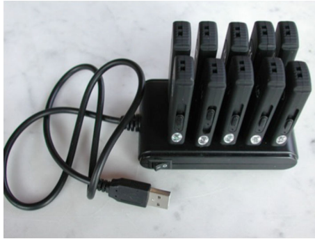
Fig. 3 Ten LRC units plugged into a USB rechargeable hub. Data contained within each unit can be downloaded and processed using this hub
