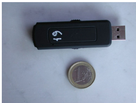
Fig. 2 The UR-09 LCR from ShenZhen HNSAT Industrial Co. Ltd (China). This miniaturized acoustic data logger can be easily deployed in the field with extend sampling times (approximately 16 h)
