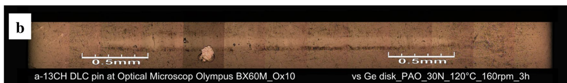
(b) a-C:H coating/germanium contact at 120°C under 30N load for 3h.
