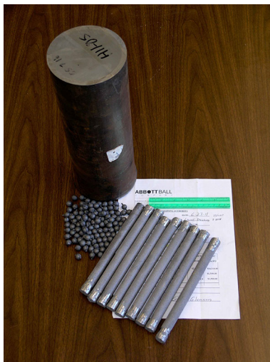
Fig. 4 60NiTi ingots and blanks produced by PM process
