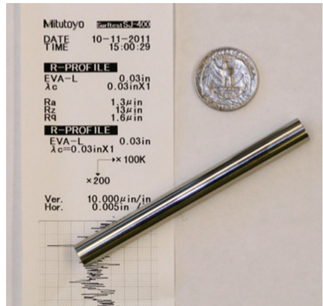
Fig. 6 Polished 60NiTi RCF rods
