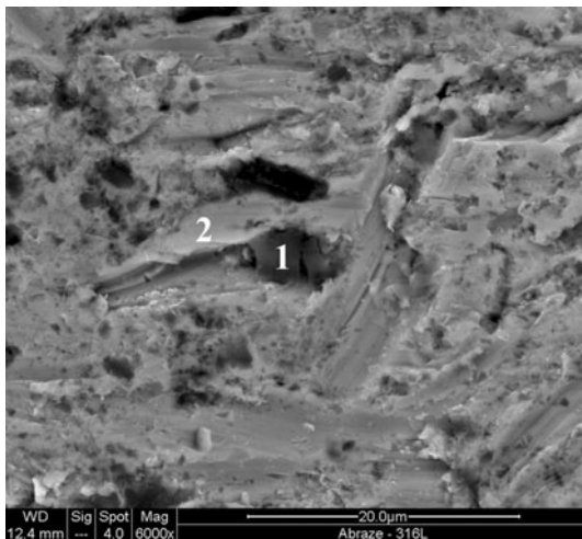
Fig. 5 Surface of AISI 316L coating after dry abrasion wear test (the embedded \text{Al}_2\text{O}_3 particle is labeled “1”, and the coating material is labeled “2”)
