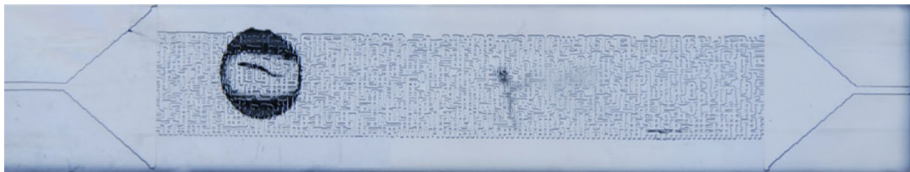
Fig. 3 The microfluidic chip before pressurizing the overburden fluid to remove the air bubbles
