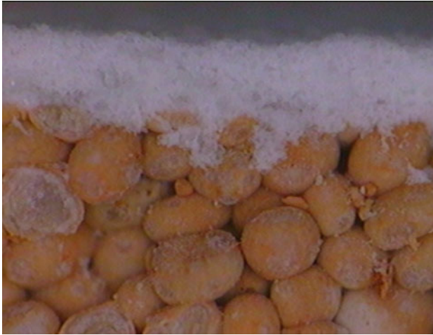
Fig. 2 Bridging with a coarse carbonate solid ( d_{50} = 40 \mu\text{m} ) on a Ketton limestone core (with pore d_{50} = 60 \mu\text{m} )
