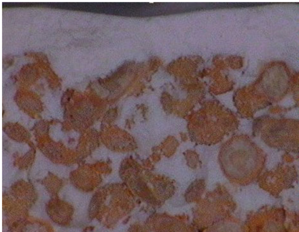
Fig. 1 Invasion of ultra-fine carbonate C1 ( d_{50} = 4 \mu\text{m} ) on a Ketton limestone core (with pore d_{50} = 60 \mu\text{m} )
