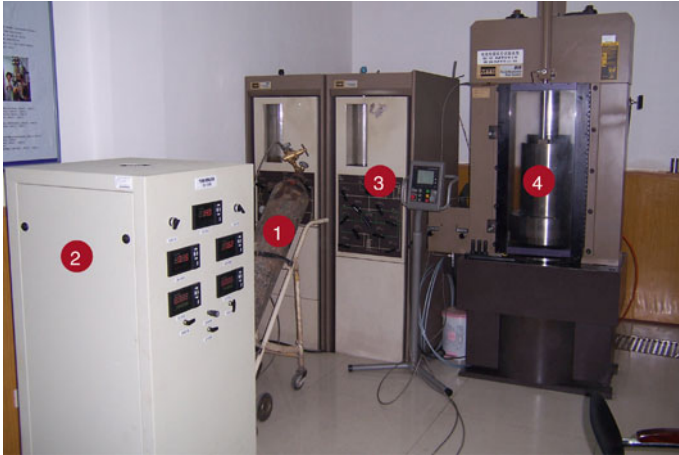
Fig. 1 Testing system of gas permeability of rock under confined pressure. Notes: (1) Nitrogen cylinder and relief valve; (2) Testing box of gas flow including flow meter, pressure difference meter and accumulator; (3) Load control cabinet; (4) MTS test platform and fractured specimen
