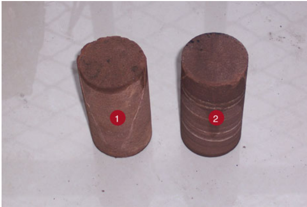
Fig. 3 Fractured sandstone specimens after uniaxial compression
