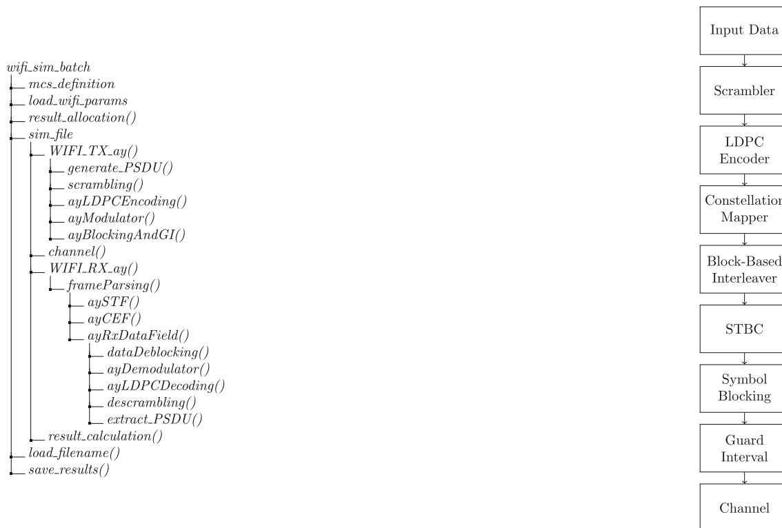
Fig. 1 Scripts and functions of the IEEE 802.11ay SC-PHY MATLAB simulator; [right] baseband signal processing chain in the IEEE 802.11ay SC-PHY transmitter (TX)
