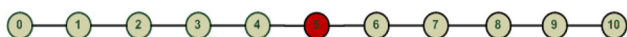
Fig. 7 A linear topology made up of 11 nodes; one of which (i.e., node 5) is a gateway
