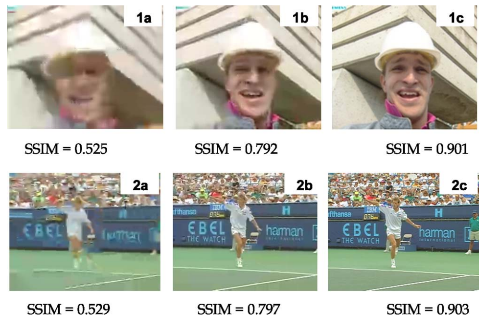
Fig. 8 Error burst with 30% frame loss for Foreman (1) and Stefan (2) video traces for the conventional H.264/AVC coding (1, 2) a , short term motion compensation references ( k = 2 ) with FP (1, 2) b and long term motion compensation references ( k = 4 ) with FP (1, 2) c
