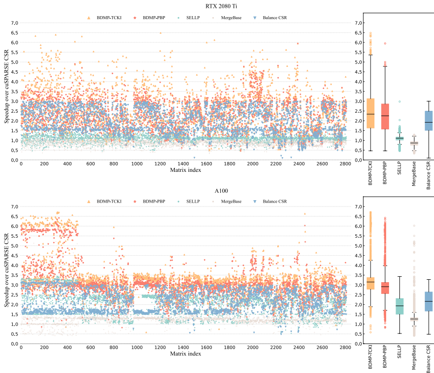
Fig. 6 Speedup of SELLP, MergeBase, BalanceCSR, BDMP-PBP, and BDMP-TCKI versus cuSPARSE CSR, as run on Turing and Ampere GPU
