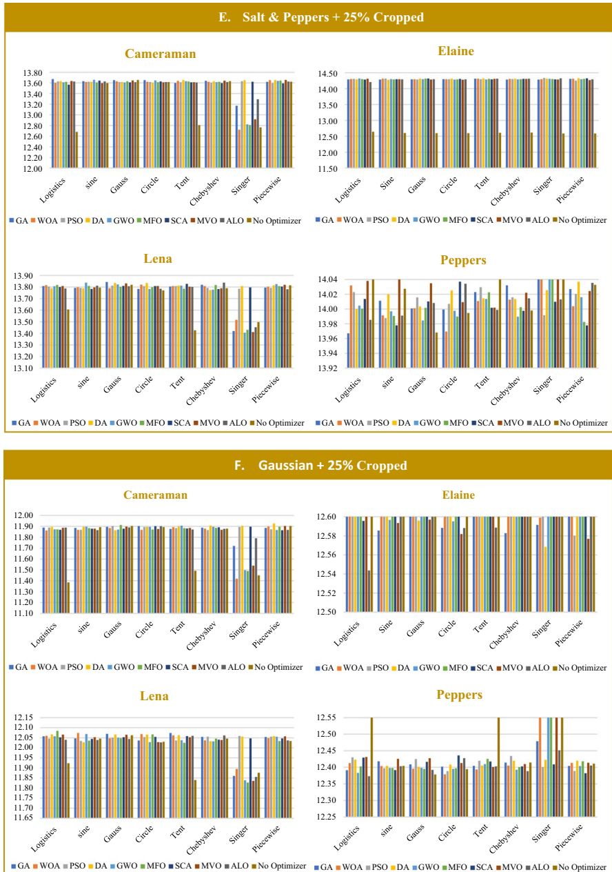
Fig. 20 Comparative analysis of PSNRs of the decrypted images after applying noise and cropping attack to the encrypted -Different Chaotic maps with different optimizers and with no optimizer
