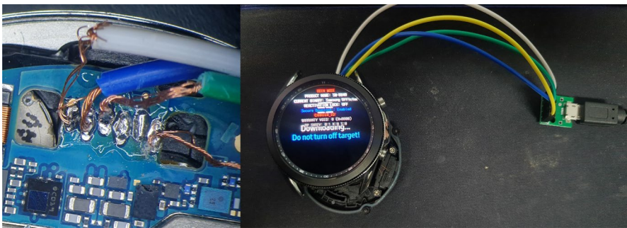
Fig. 4 Soldering to Galaxy watch 3 PCB service port using standard wire
