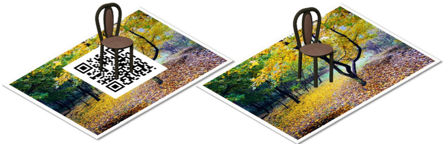
Fig. 1 Augmented reality using marker (left is binary marker and right is image marker)
