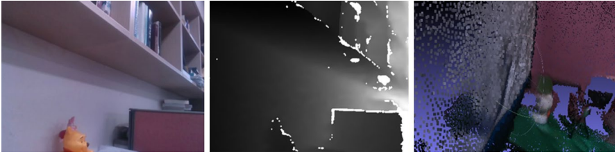
Fig. 3 Example of input data and point cloud (left: RGB image from the real world, middle: depth image from the real world, right: generated point cloud)
