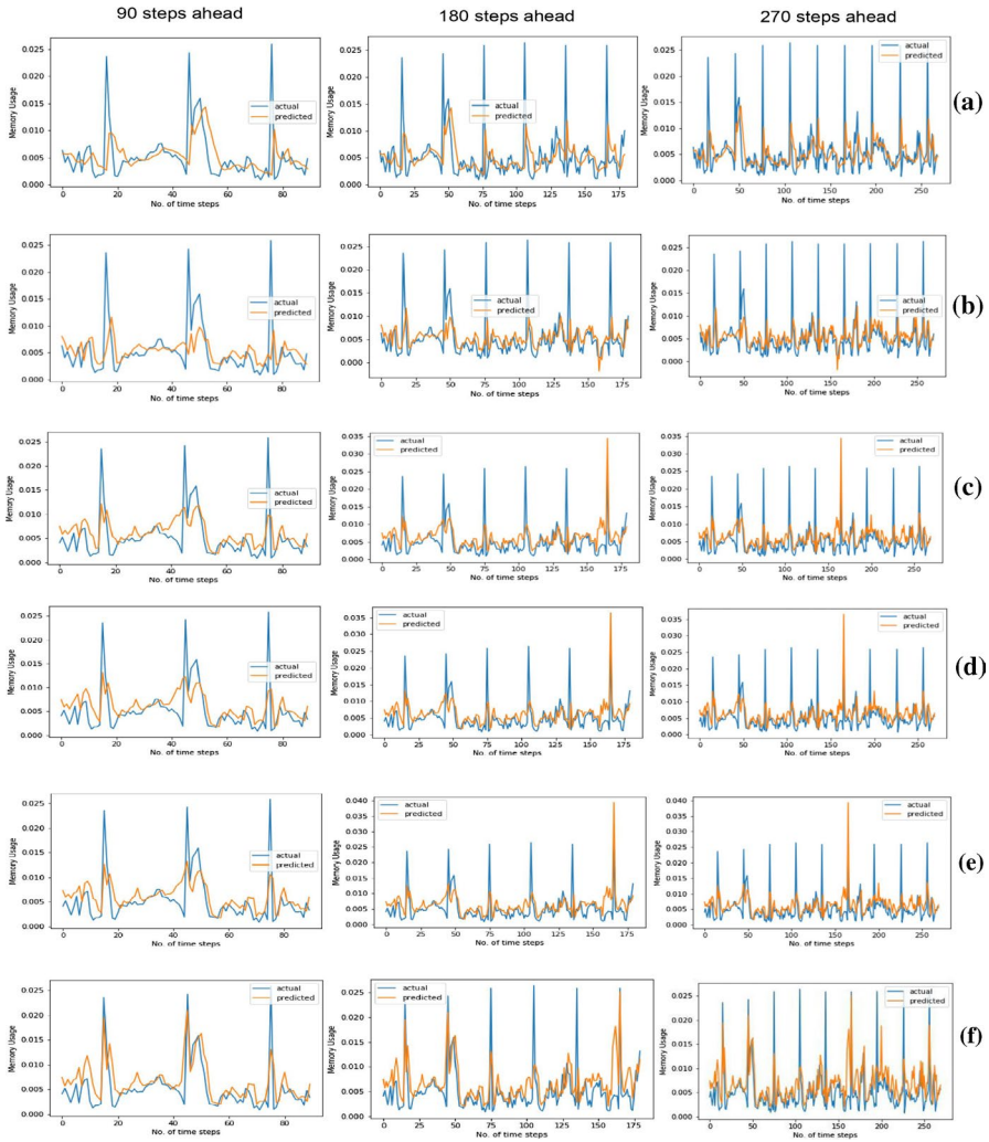
Fig. 14 Multi-steps-ahead memory prediction with all features using a ARIMA, b Linear Regression, c GRU, d LSTM, e BiLSTM, f Clustering-based Stacked BiLSTM
