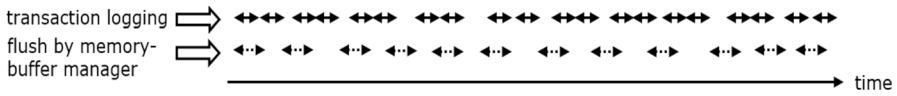
Fig. 10 Metadata disk usage over time when our memory-buffer manager mechanism is applied
