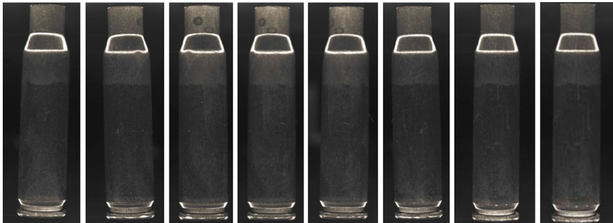
Fig. 3 Images covering the entire 360-degree (8x45 degree) surface of the same military case
