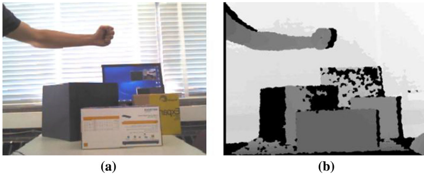
Fig. 1 Example of a Kinect dataset a color image, and b depth map (color figure online)
