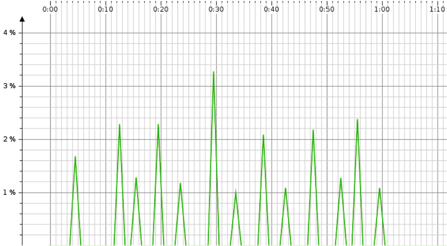
Fig. 13 Garbage collection overhead in Terasort (SSD + SSD configuration) using JVM reuse option. In this figure, the x-axis shows the elapsed time (min) and the y-axis shows how much time (%) was spent for garbage collection
