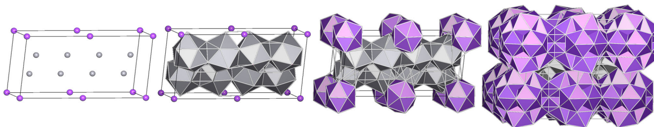
Fig. 4 Formation of the \text{Ho}_6\text{W}_4\text{Al}_{43} structure with nanoclusters: The gray balls (Al6) are the centers of icosahedra, and the purple balls (W2) are the centers of Mackay clusters (Color figure online)
