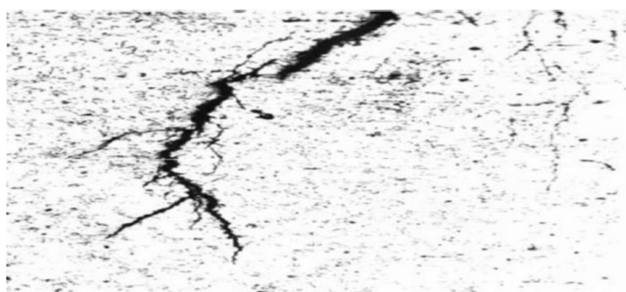
Fig. 5. Intercrystalline crack in 08KhMChA steel ( \times 100 ).
