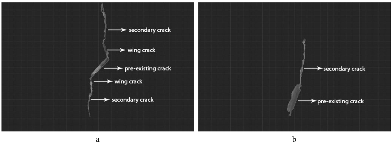
Fig. 6. The failure and fracture patterns of cubic concrete specimens with a single centered crack at different inclination angles.
