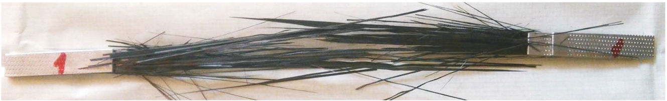
Fig. 2. Specimens of CFRP with longitudinal reinforcement after tensile testing at room temperature.
