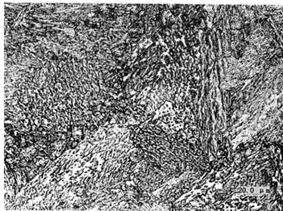
Fig. 3. SEM illustration of the cross-section of the nitrided layer.
