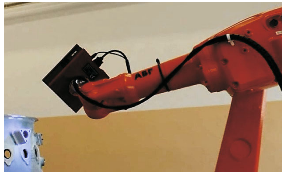
Fig. 8. The chamfer is measured with the 3D scanner.
