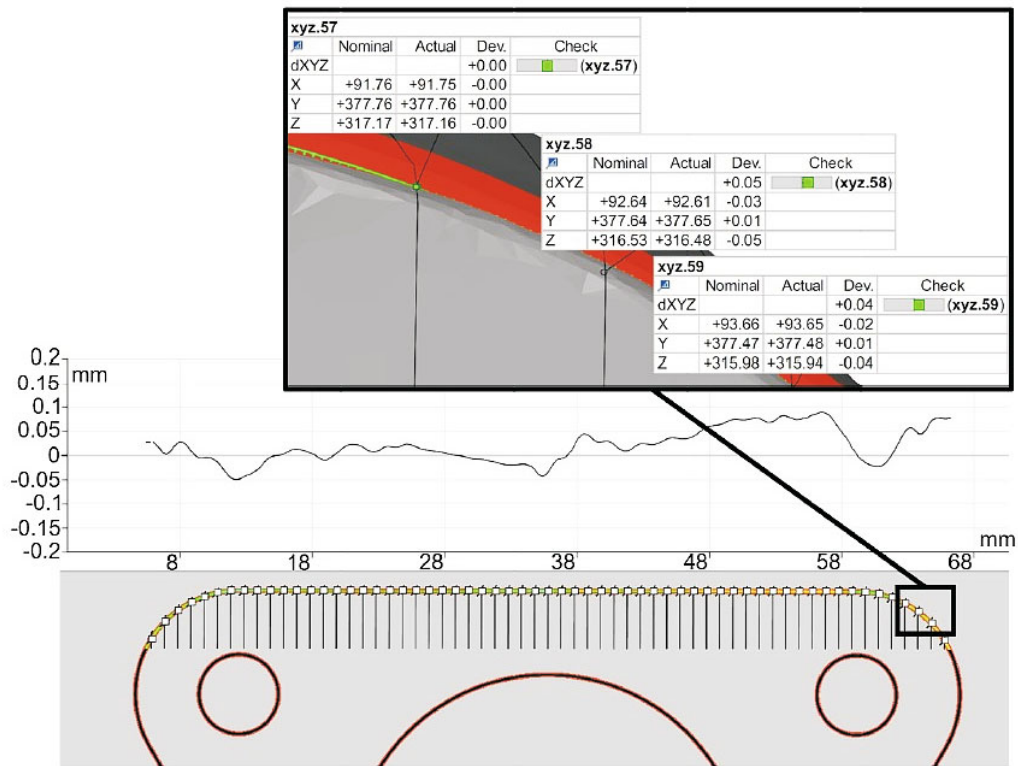
Fig. 12. Produced chamfer accuracy changes vs. tool path. (Three-cornered boss top edge, measurement No. 16.)
