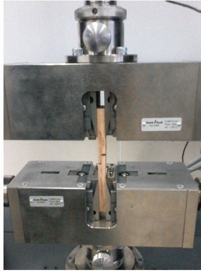
Fig. 1. Experimental design for bonding strength tests.
