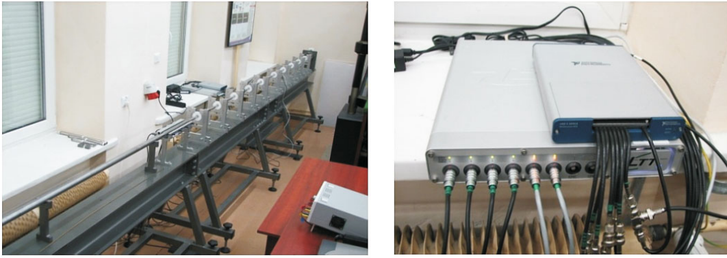
Fig. 4. A perspective view of the SHPB apparatus for testing materials at high strain rates (SHPB = split-Hopkinson pressure bar).
