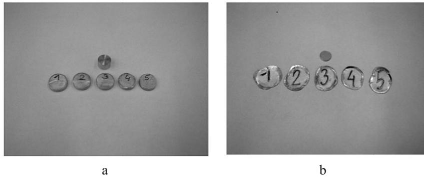
Fig. 11. Exemplary specimens of 1050A aluminum after dynamic compression test at high strain rates: (a) D=10 mm, L=5 mm; (b) D=10 mm, L=1 mm.
