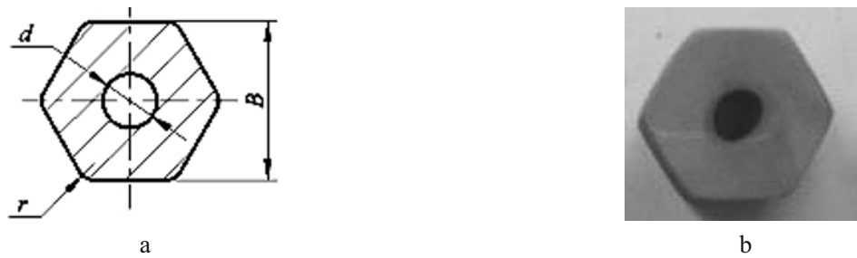
Fig. 1. Scheme (a) and photo (b) of the drill steel specimen cross section (B22 type drill steel: B = 22 mm, d = 6 mm, and r = 2 mm).
