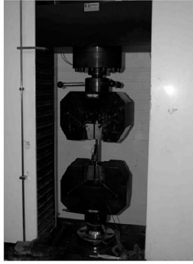
Fig. 1. Tensile testing machine.
