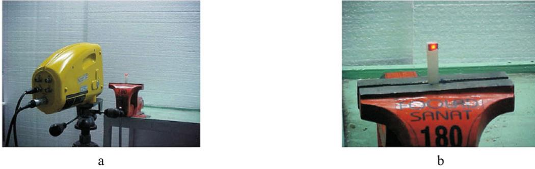
Fig. 1. Vibration measurement by laser doppler vibrometer OMETRON VH300+ (a) and specimen (b).
