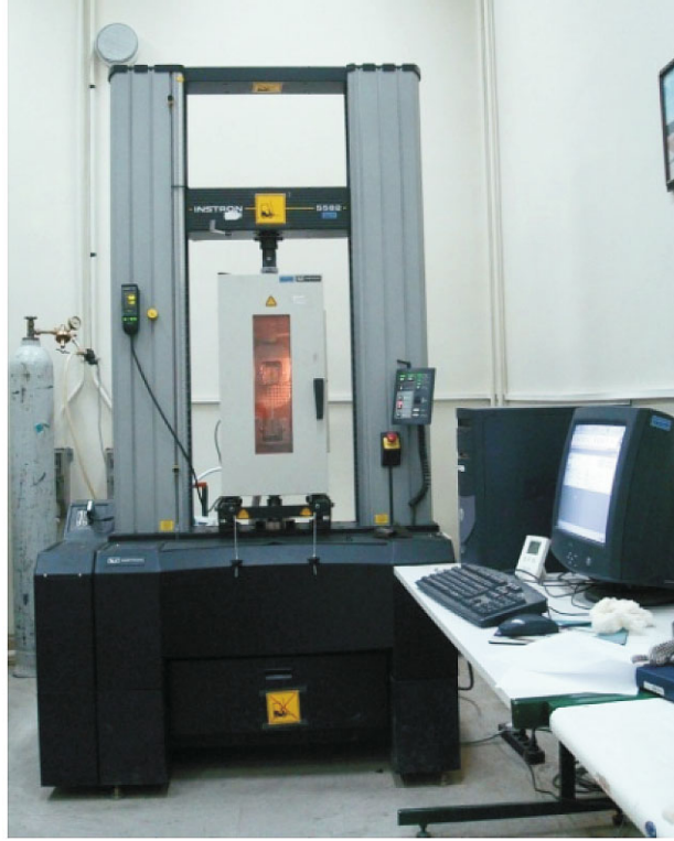
Fig. 3. Experimental set up for mechanical testing at room and low temperatures.
