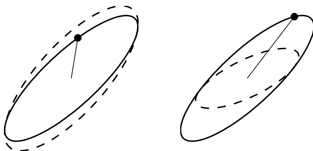
Fig. 1 Two examples of the RAM update (R3). The solid line represents the contour ellipsoid defined by S_{n-1}S_{n-1}^T , and the vector S_{n-1}U_n/\|U_n\| is drawn as a dot. The contours defined by S_nS_n^T are dashed
