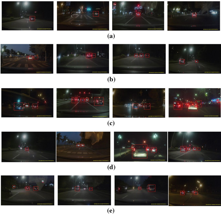
Fig. 13 Examples of detection results with proposed method. a Single and b multiple vehicles detected with the proposed method. c Vehicles detected accurately under complex backgrounds. d Blurred and e partly occluded vehicles are also detected, although f some results missed vehicles or produced false positives
