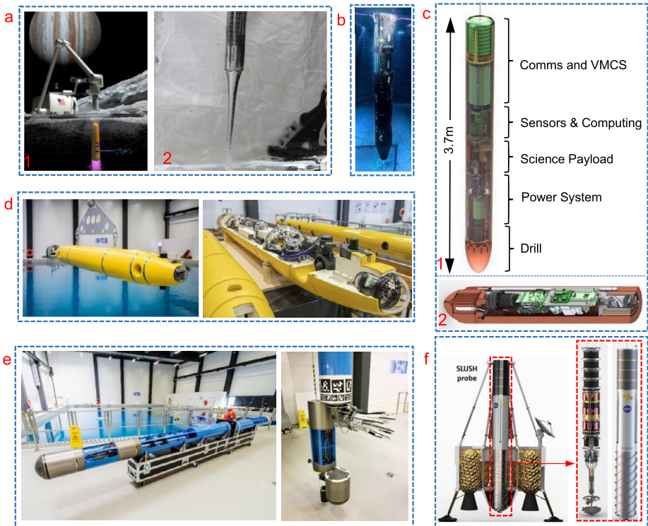
Fig. 12 Terrestrial ice penetration drills. (a) ARCHIMEDES ice cavern robot: 1-Concept of terrestrial ice penetration drills; 2-DLP tested in an ice block. (b) THOR. (c) PROMETHEUS project: 1-PROMETHEUS cryobot; 2-CCHWD. (d) DeepLeng. (e) Teredo IceShuttle. (f) SLUSH
