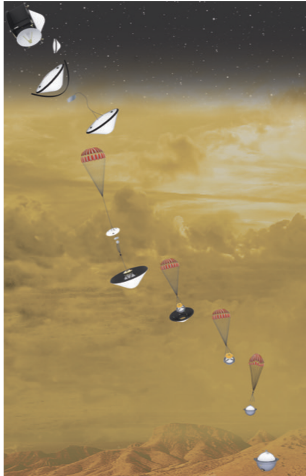
Fig. 10 The NASA DAVINCI mission (Garvin et al. 2022) will conduct in situ sampling of the Venus atmosphere during its \approx hour-long descent to the surface, providing critical measurements of noble gases and stable isotopes
