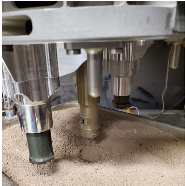
Fig. 46 Regolith sampling with the EDU Corer in a Mars soil simulant
