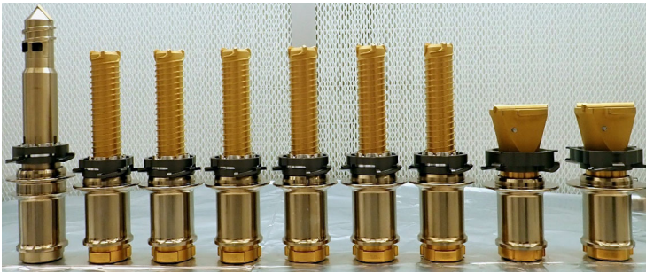
Fig. 17 Set of flight Bits stored in the Bit Carousel. From left to right, 1x Regolith Bit, 6x Coring Bits, and 2x Abrading Bits. Note the Launch Abrading Bit (installed in the Corer Chuck for launch) is not shown here
