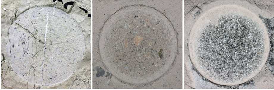
Fig. 47 Examples of rock abrasions after gDRT dust removal. Left image is KMM, middle image is BTI, and right image is USB rock
