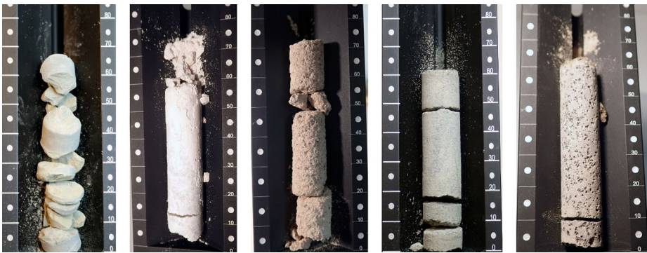
Fig. 48 Examples of rock cores collected in QMDT. Rock types from left to right: KMM, CRG, BTI, NBS, and USB
