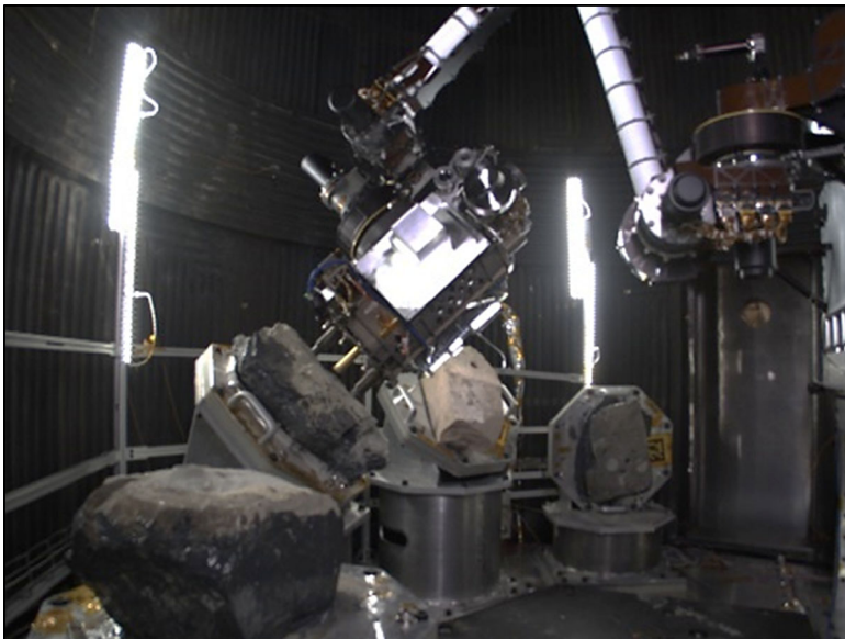
Fig. 44 QMDT testbed inside the 10 foot chamber with several geoanalog rocks mounted on pedestals in different orientations. Turret/Corer and Robotic Arm are visible in the center of the image
