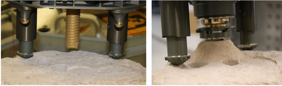
Fig. 16 Example of coring in a test rock article with the qualification model Corer. The left image shows the Stabilizers conforming with the rock surface and the Coring Bit prior to advancing. The right image shows the Chuck and Bit position at the bottom of the drilling operation, with rock cuttings powder coming out of the drill hole
