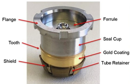
Fig. 37 Ground test Seal (left) with the component parts labeled. Flight Seal Assemblies shown in different orientations (right images). Middle image has the side that is inserted into the Tube facing up. Each Seal is uniquely serialized
