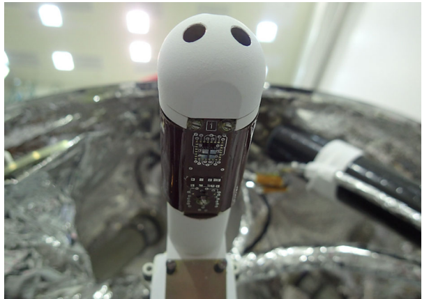
Fig. 19 Details of TWINS' Wind Sensor. View of the bottom board, with the four dice at the close tip, and the cold die at the far end
