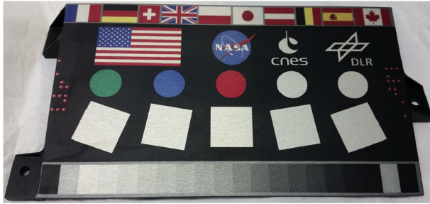
Fig. 12 InSight camera calibration target. The top face of the target is 17 cm by 10 cm in size. The flags on the calibration target represent the nations that were directly participating in the InSight mission as of late 2014 (when the design of the calibration target was frozen). They are (top row, from left to right): France, Germany, Switzerland, United Kingdom, Poland, Japan, Austria, Belgium, Spain, and Canada. The second row from top contains the flag of the United States of America, the NASA logo, Centre National d'Etudes Spatiales (CNES) logo, and Deutsches Zentrum für Luft- und Raumfahrt (DLR) logo. The third row from the top contains dots for color and geometric calibration. The fourth row contains slanted square edges for sharpness (MTF) measurements. The fifth row contains a greyscale intensity ramp for signal/noise measurements
