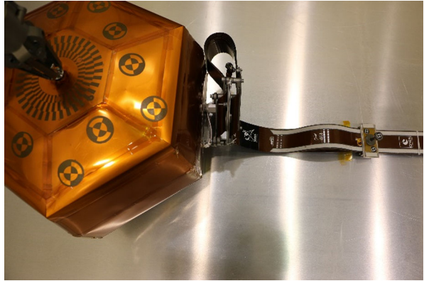
Fig. 15 SEIS Tether with LSA Service Loop and Pinning Mass
