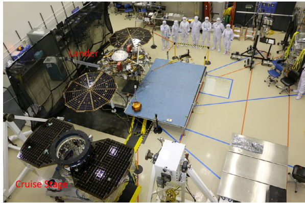
Fig. 1 InSight Spacecraft Lander and Cruise Stage at Lockheed Martin Space Facility in Littleton Colorado
