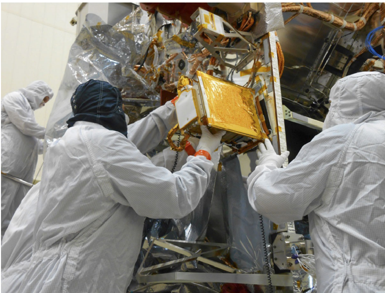
Fig. 13 REXIS instrument mounted onto the OSIRIS-REx spacecraft, December 18, 2015
